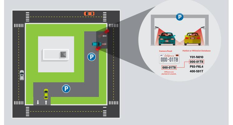
ELSAG fixed plate reader cameras installed at all access points read license plates and capture a photo of the vehicle, date and time stamps, plus vehicle make, type, and color. Simultaneously, each plate number is compared to databases of license plates to validate permits and sessions and to identify vehicles associated with scofflaw activity, in which case enforcement officials are alerted in real time.
